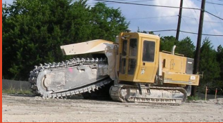
Bucket-chain trencher
