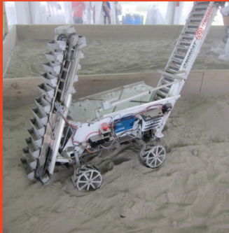
Bucket-chain trencher
