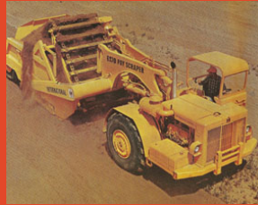
Elevating scraper
