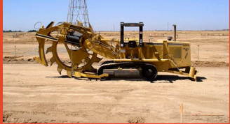
Bucket-wheel trencher
