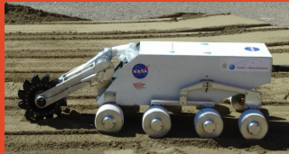
Bucket-wheel trencher
